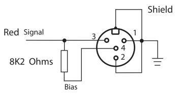
Note, mic boom must be grounded to shield
